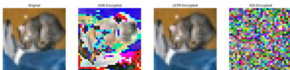
FIGURE 4. Comparison of Original, GAN Encrypted, LSTM Encrypted, and AES Encrypted Images
